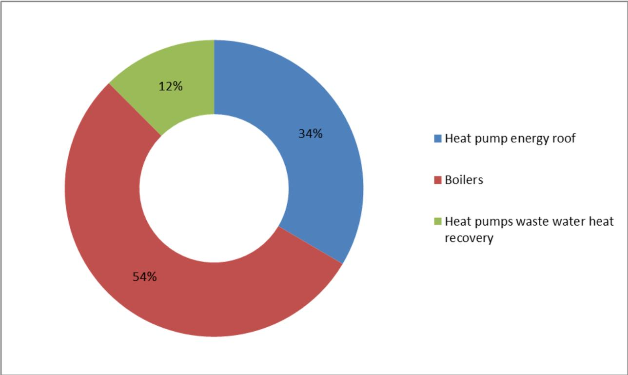
Fig.5 Monitoring data on the heat supply for Nekkerpool
