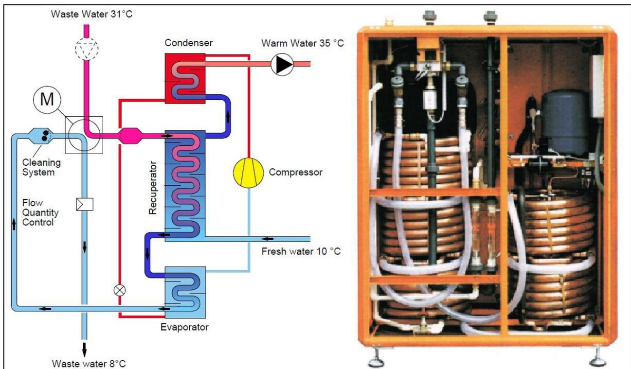
Fig.3 Waste water heat recovery unit with recuperator and heat pump
