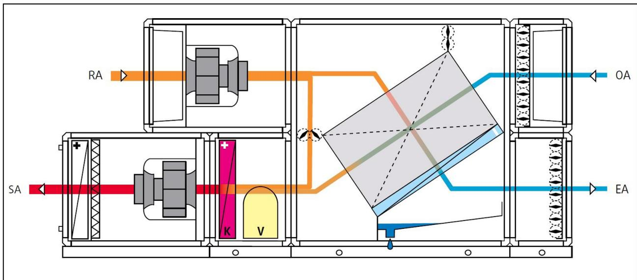
Fig.4. Air handling unit with integrated heat pump (evaporator in blue, condenser in red, compressor in yellow) for climatisation of the swimming pool hall
