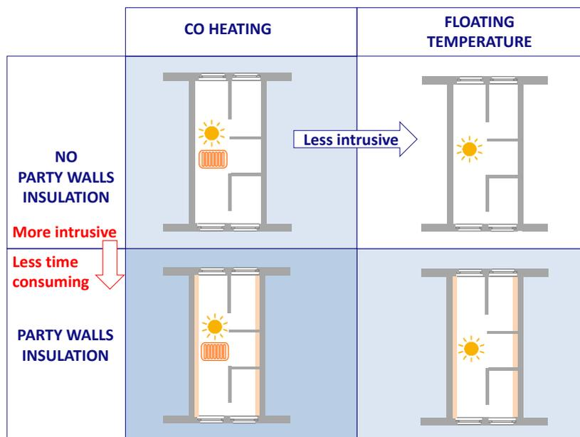
**Fig. 2** Different boundary conditions and heat sources for the measurement of the Heat Loss Coefficient.
