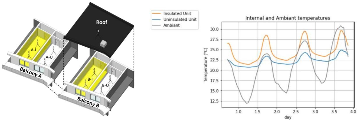
**Fig. 3** Measured floating temperatures with and without insulation panels covering the party walls of identical units (Printemps, Brussels, 2017/05/24-2017/05/27).
