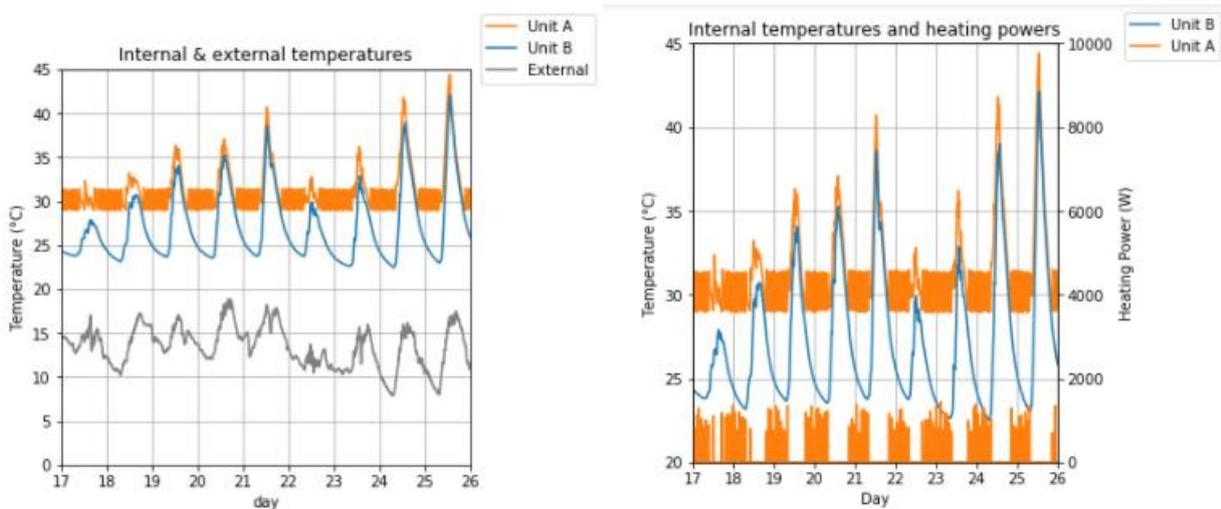
**Fig. 5** Evolution of external temperature and internal temperatures in two identical units provided with inside insulation, B in floating temperature mode and A in co-heating mode (left) and evolution of the heating power in unit A (right).
