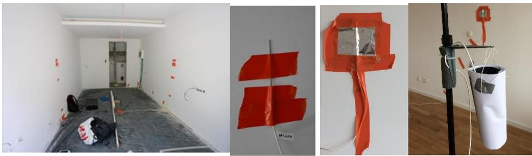
**Fig. 4** Temperature measurement at the interface of insulation layer before placement of insulation panels (left, center left) and at the surface of uninsulated walls (center right) and air temperature probe (right).
