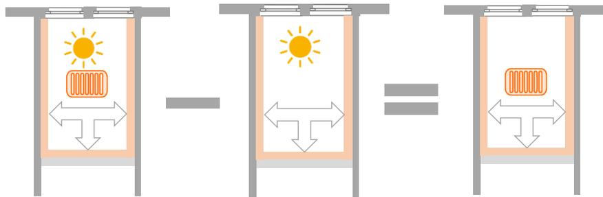
**Fig. 6** Analysis process considering the temperature difference between two identical units provided with inside insulation panels: one of the unit is co-heated while both are submitted to identical solar heat gains.
