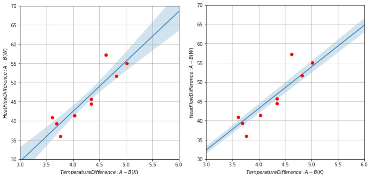
**Fig. 7** Correlation between daily mean heat power differences and temperature differences between two identical insulated units, without (left) and with (right) forced intercept.
