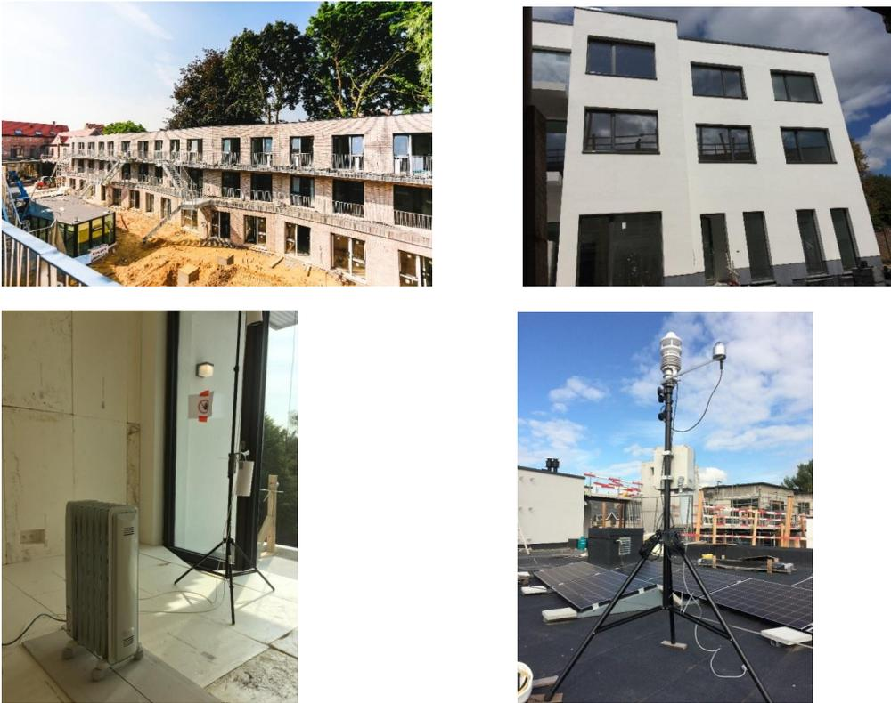
**Fig. 1** Measurements sites: student dwellings in Etterbeek (up left), apartments in Neder-over-Heembeek, Brussels (up right), experimental setup inside the units with insulation panels, electric radiator, internal air temperature sensors and external pyranometer on the balcony (down left), weather station located on the roof (down right).
