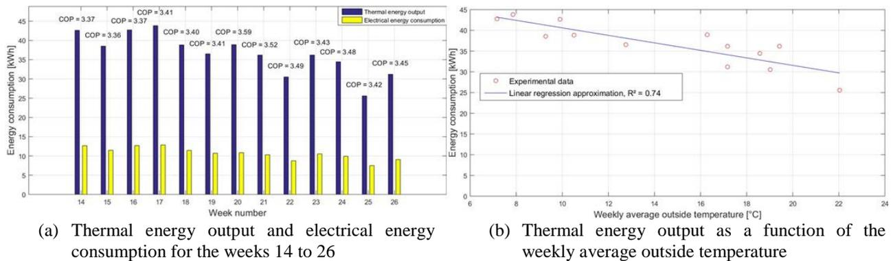
**Figure 3:** On-site performance of the heat pump in domestic hot water production mode
