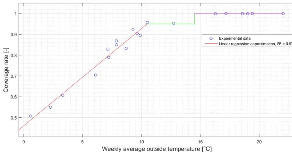
**Figure 6:** Coverage factor of the heat pump as a function of the weekly average outside temperature
