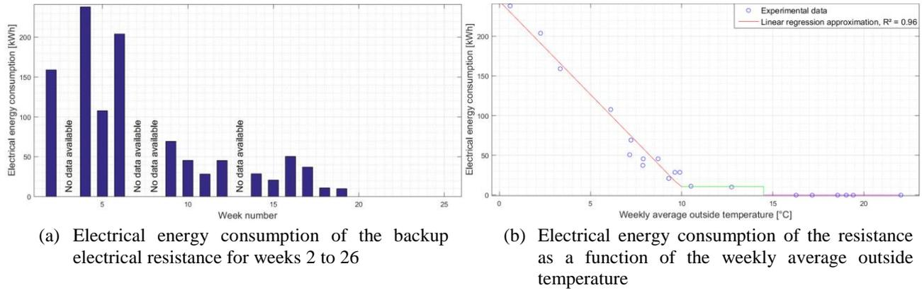
**Figure 4:** Energy consumption of the backup electrical resistance on a weekly basis
