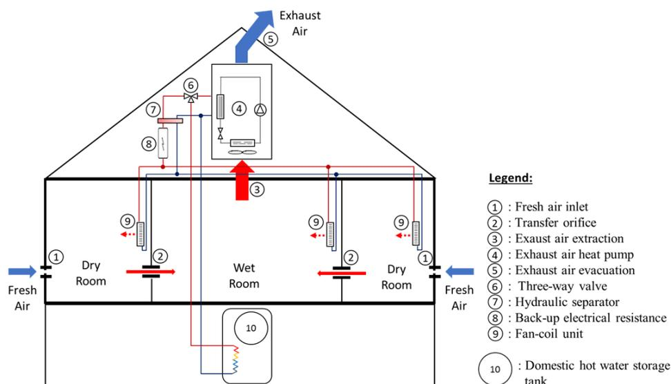
**Figure 1:** Simplified representation of the HVAC systems
