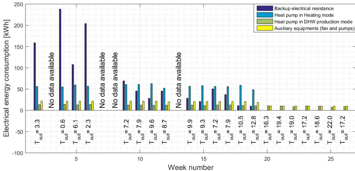
**Figure 5:** Electrical energy consumption of the backup electrical resistance, the heat pump in heating mode, the heat pump in DHW production mode and the auxiliary equipment on a weekly basis
