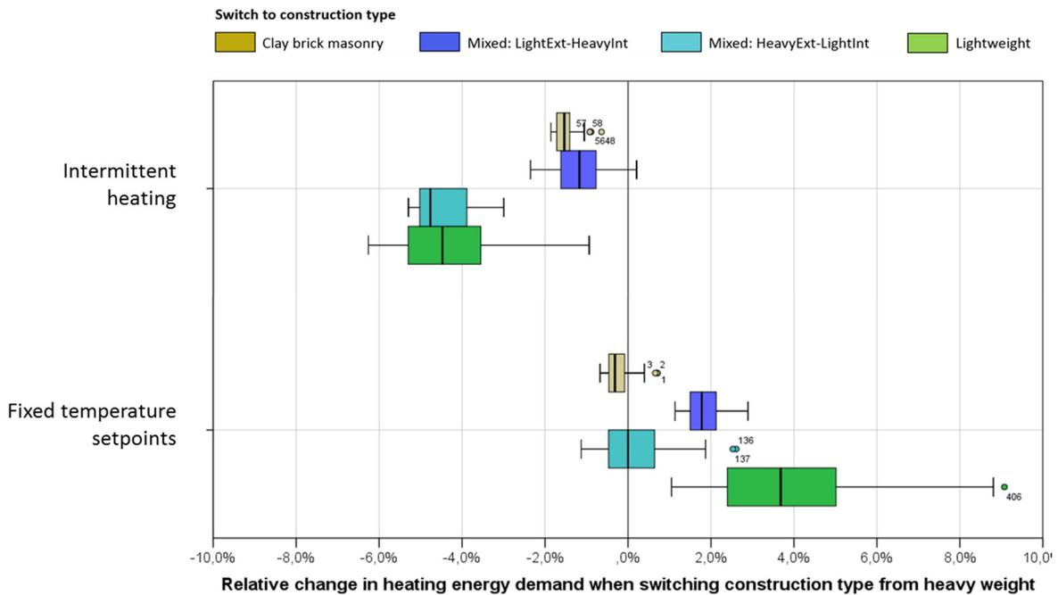
**Fig. 3** Relative change in annual heating demand when switching construction type from heavy weight to different variants with less thermal inertia – in relation to distinct heating schedules.
