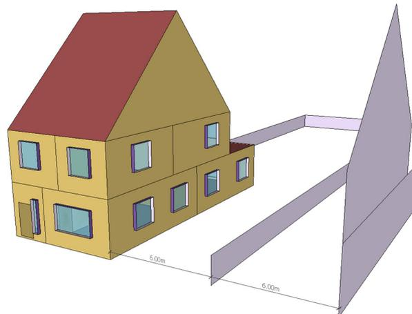
**Fig. 1** Building geometry rendering, including external shadow casting objects and window reveals
