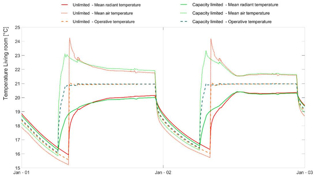
**Fig. 4** Time series data for capacity limited HVAC system with early start-up versus unlimited power (semi-detached heavyweight dwelling with R5 insulation, standard double glazing and medium glazed area)
