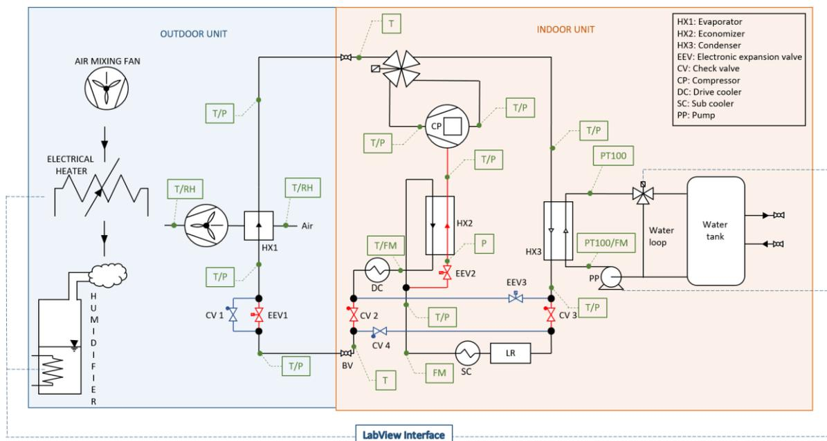
Fig. 1 Experimental set-up scheme.
